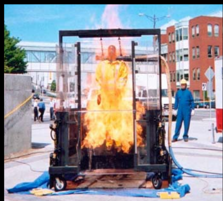
Flame resistance testing on PSP's FIREWALL™ Rainwear used by workers in the utility and petrochemical industries.
