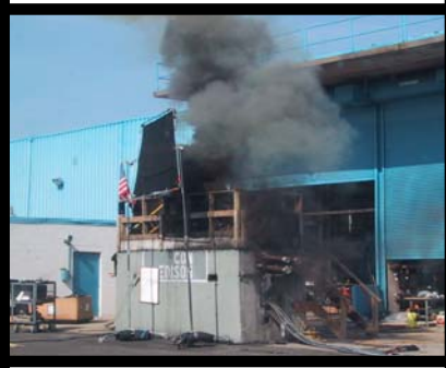
AEGIS EXPLOSAFE™ manhole blast/arc simulation testing.
